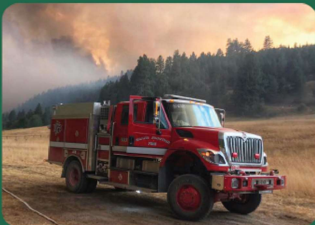
Brush 4 is huge, the tires alone are nearly four feet tall to give it high clearance for rugged terrain
