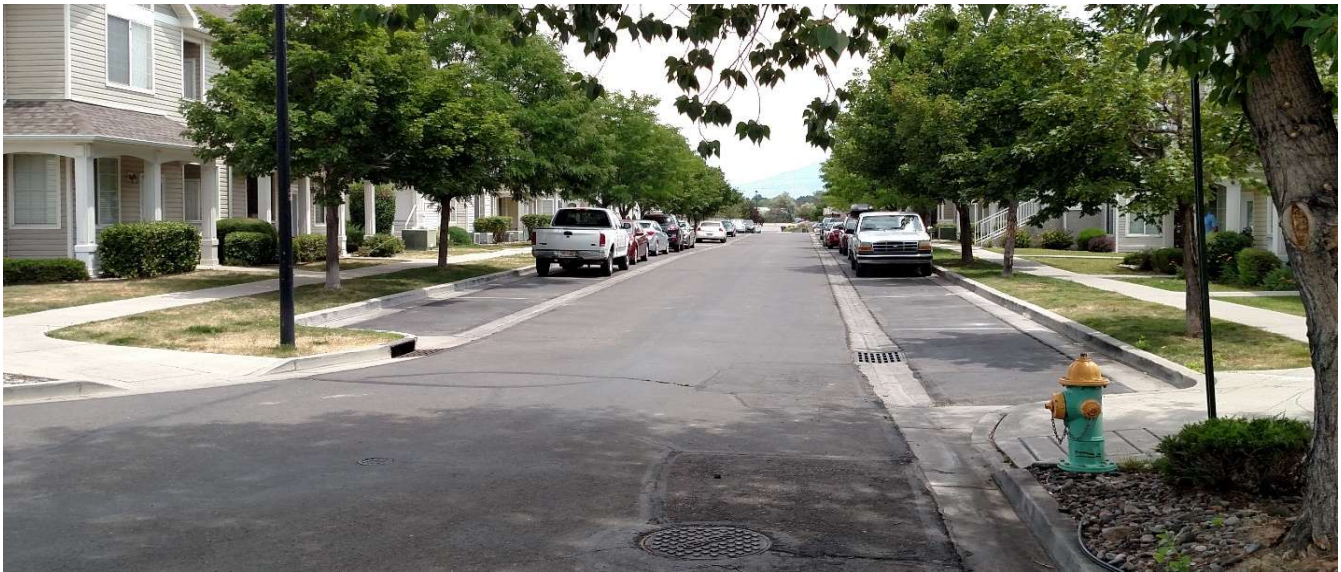
Inset Parking and Valley Gutters – Extending curbs out at intersections and midblock with inset parking can help the street feel narrower encouraging safer speeds while maintaining street parking and emergency access widths. Valley gutters between street parking and travel lanes slope towards one another creating a narrow feel.
